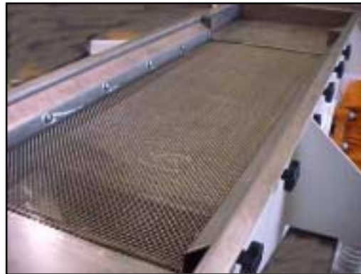
◀ Twin rotary vibratory screen illustrating quick change screen for easy cleaning and optimum sanitation.
